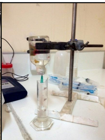
Figure3. Gas collection by displacement.
