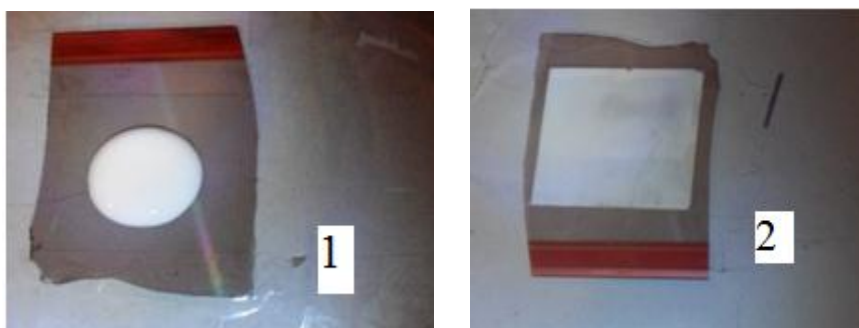
Figure3. Applying the film of \text{TiO}_2 to the ITO glass.
