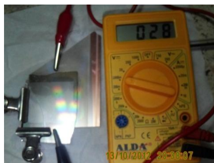
Figure 7. The solar cell subjected to a light source.
