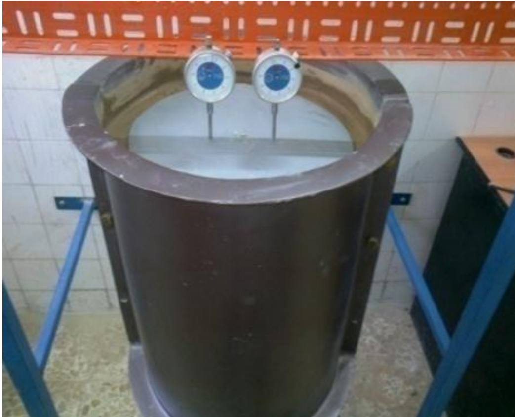
Figure 3. Plate of (GPA-Foundation System) under the heave.
